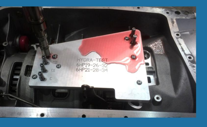
This is a favourite tool of so many customers. Described by some as the "must have" tool for all transmission rebuild shops. By flow checking individual clutch circuits within the transmission unit, damaged seals or even piston cracks can be detected. The system is so portable it can be performed anywhere in your workshop.
