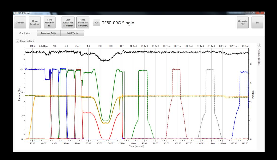
The Hydra-Test Controller functions as the "brain" of the entire system. Its accuracy and stability now make our system a complete and reliable package HTC-K<sup>™</sup> Controller and software provides precise and easy to analyse graphics.
